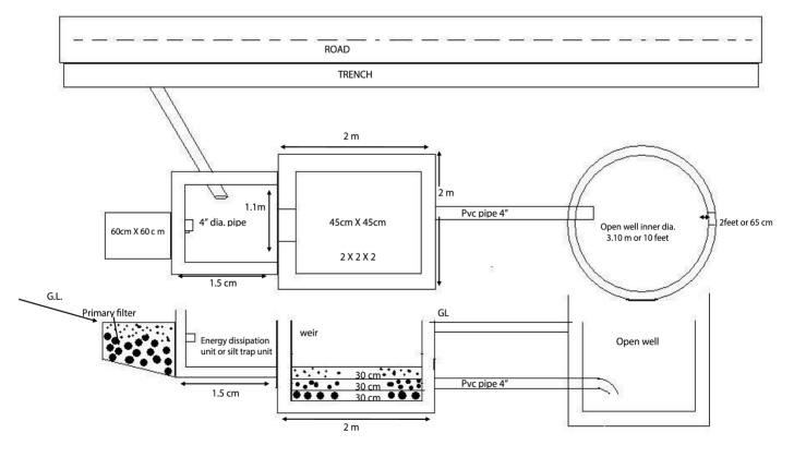
Fig. 1 : Schematic diagram of artificial well recharging system
